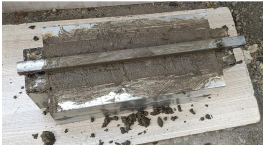
Figure 12. Casted concrete hollow block.
