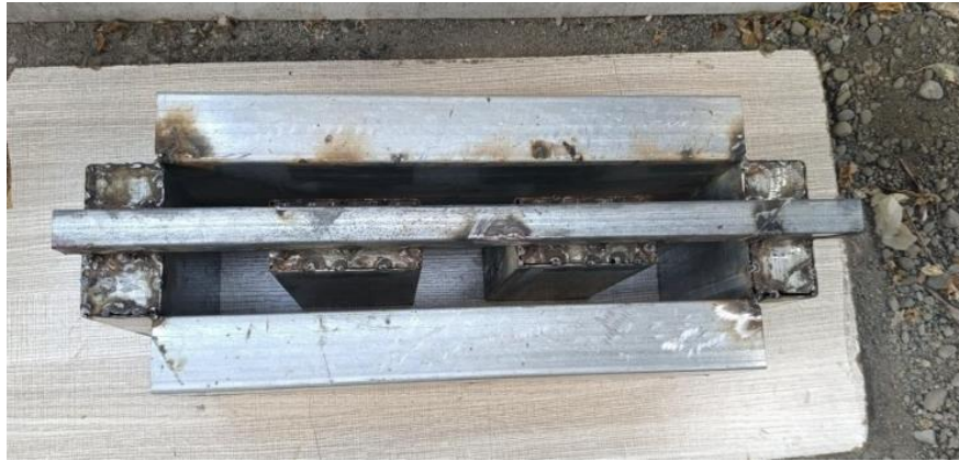
Figure 11. 100mm x 200mm x 400mm steel hollow block mold.
