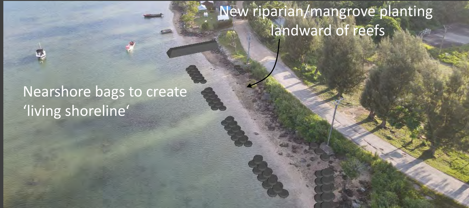
Nearshore: Coastal reefs for wave protection
